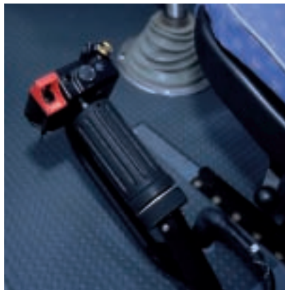
Fuel flow twist grip on pilot stick
