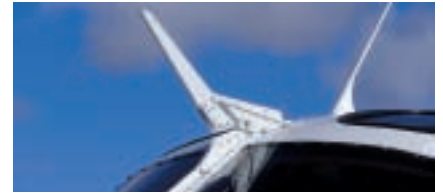
Cable cutter for wire strike protections
