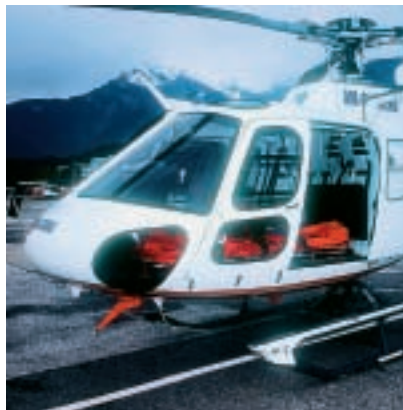
Upper & lower cable cutters for wire strike protection
